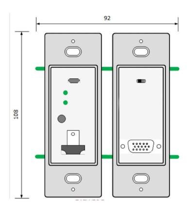
All measurements in millimeters (mm)
