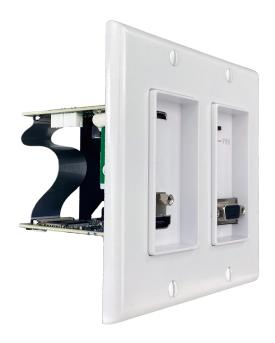
The Ultra Series 717WP2 Wallplate Encoder (Transmitter) fits into a 2-gang construction box and provides HDMI, VGA, and line audio inputs to any Just Add Power video distribution system. Distribute 4K video over a Cat5e or greater network cable.
