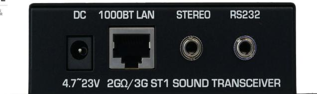
**Operates as either a Transmitter or a Receiver.**
