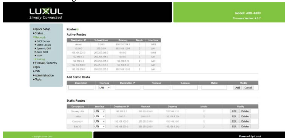
Static Routing on a Luxul ABR-4400
